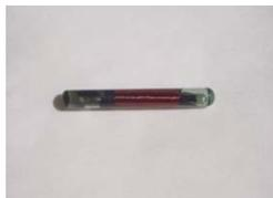
Figure 8 : Transpondeur TIRIS (Texas Instrument Radio Identification System)
